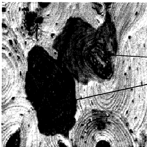
Fig. 1A 400 MHz (120 aperture, burst mode) SAM micrograph (resolution approximately 2.5 \mu\text{m} ) of a portion of human femoral cortical bone cut transverse to the bone axis. The two center osteons show darker gray levels than does the surrounding bony tissue.
